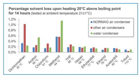
In a direct comparison, the air cooler from NORMAG shows a significantly lower solvent loss than other air coolers. This difference is particularly clear for shorter periods of use.
